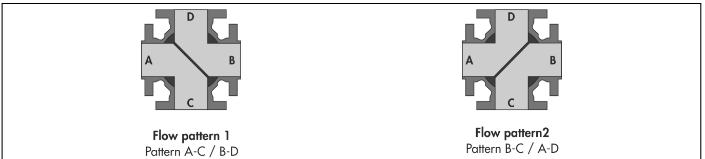
Fig. 5: Flow patterns for BR 26x 4-way Ball valve with L-port
