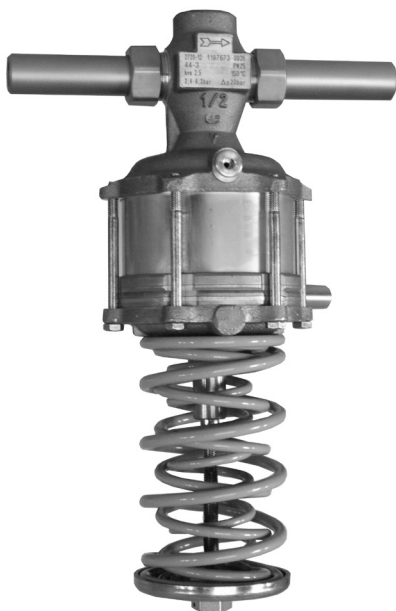
Type 2443 Safety Shut-off Valve (SSV) with integrated pressure reducing valve Red brass body with screwed ends
