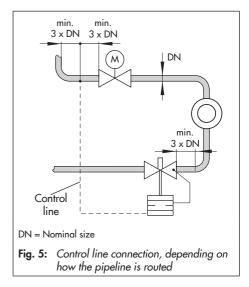
We recommend installing the control line for tapping pressure from the pipeline at a distance of at least three times the nominal size (DN) away from any pipe fittings (e.g. manifolds, bends, branches or other valves), that may cause turbulence in the flow.
