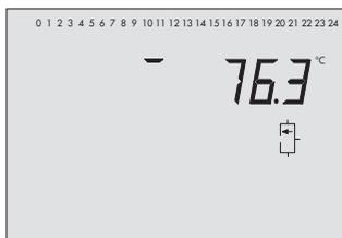
Temperatur am Speichersensoren SF2, SF3 (Pufferspeicher)
