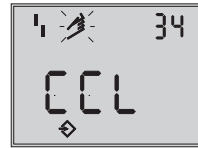
Closing direction (direction of rotation causing the valve to move to the CLOSED position (view onto positioner display) Default: CCL (counterclockwise)
